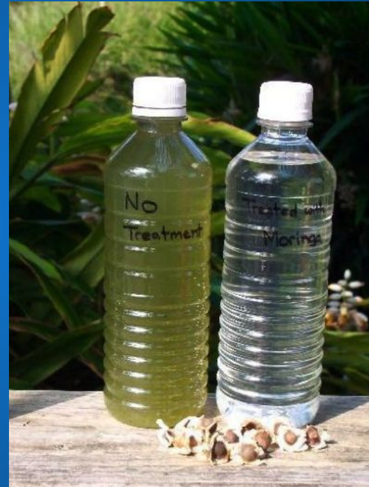
Figure 13: Water Treatment Using Moringa Seeds [7]
