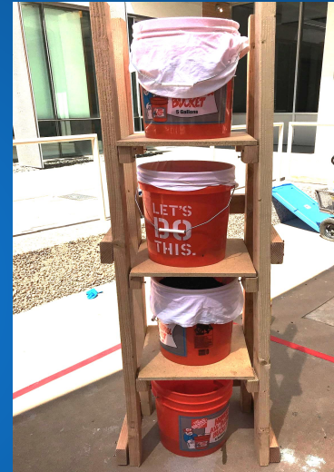
Figure 14: Constructed Water Treatment System at PSWC 2018 (Photo Courtesy of Cameron Rhodes)
